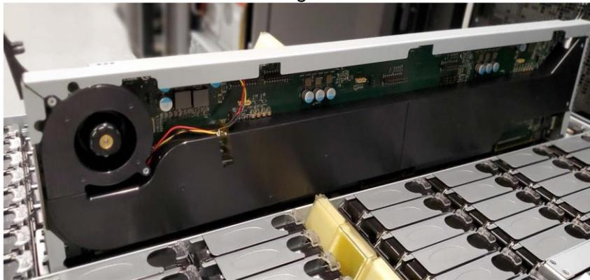
Figure 3.17 Correctly installing the IOM
