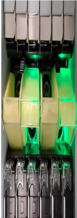
Figure 6.19 Correctly oriented PSUs
