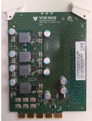
Figure 4.2 5V DC regulator board
