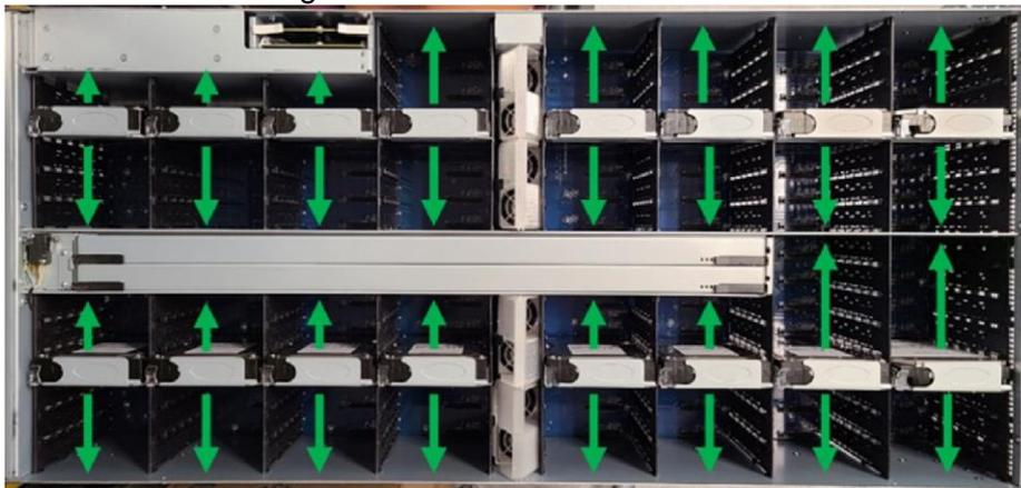
Figure 3.14 Example of drive installation sequence
