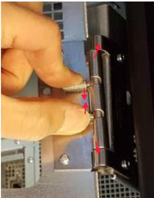
Figure D.4 Spring-loaded quick release hinge
